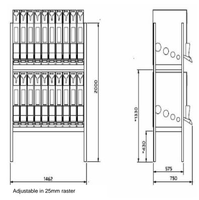
Dimensions for a storage rack with 20 masterbatch containers
