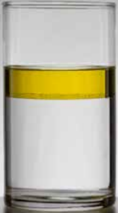
water contaminated with diesel
