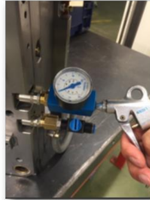
A check valve prevents the retreat of the injected compressed air.
